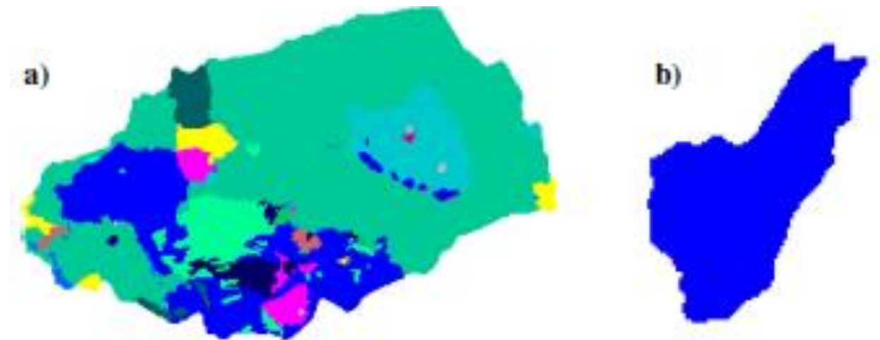
Definition of particles and grains: a) PARTICLE consisting of various grains b) Particle consisting of one GRAIN. Image from Sandmann, 2015
