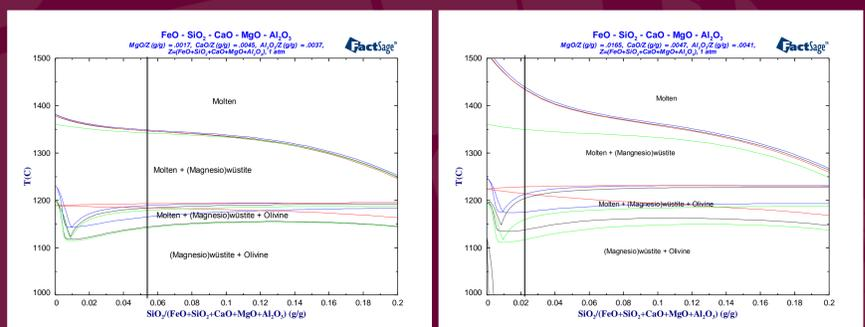
Figure 1. Phase diagrams for FeO-SiO<sub>2</sub>-CaO-MgO-Al<sub>2</sub>O<sub>3</sub>-system illustrating the melting behavior of acid (left) and olivine (right) pellets: Black lines = All five components included in the system. Blue lines = Al<sub>2</sub>O<sub>3</sub> excluded. Red lines = CaO excluded. Green lines = MgO excluded.
