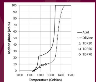
Figure 2. Comparison between computational molten phase fractions and experimental TDP values.
