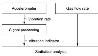
Fig. 3. Schematic illustration of signal processing and statistical analysis of the vibration indicator and the gas flow rate.
