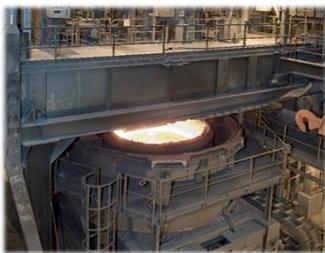
Fig. 1. Open vacuum tank with a ladle inside.
