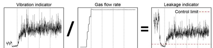
Fig. 5. Definition of the leakage indicator with a control limit.
