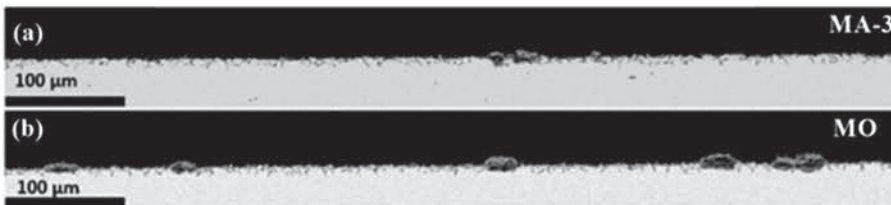
Fig. 13. Surface of AISI 309 after 5 minutes annealing at 1200 °C using different atmospheres: a) MA-3 and b) MO. (Modified under Creative Commons CC BY 4.0 license from Publication II © 2021 Authors).
