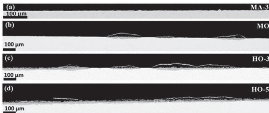
Fig. 9. Surface of AISI 304 after 5 min annealing at 1100 °C using different atmospheres: a) MA-3, b) MO, c) HO-3, and d) HO-5. (Modified with permission of Wiley-VCH GmbH from Publication III © 2022 Wiley-VCH GmbH).
