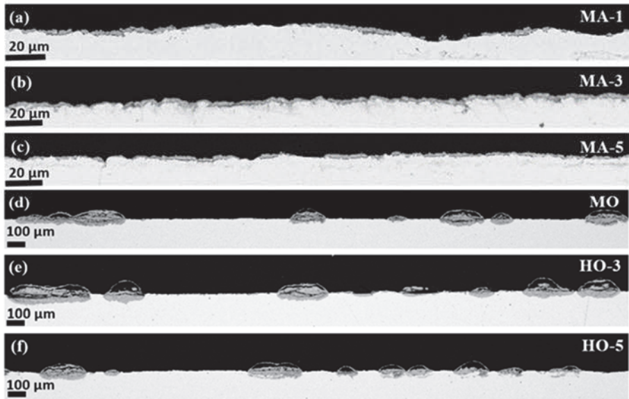
Fig. 14. Surface of AISI 441 after 5 minutes annealing at 1100 °C using different atmospheres: a) MA-1, b) MA-3, c) MA-5, d) MO, e) HO-3 and f) HO-5.
