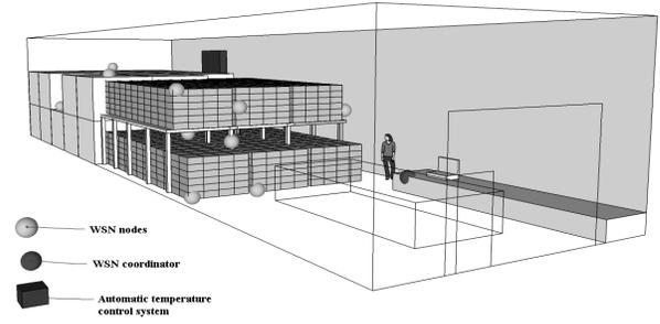
Figure 9. WSN for remote environment monitoring installation inside the warehouse
