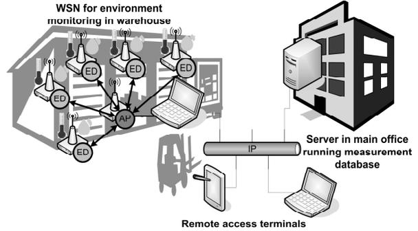
Figure 10. Architecture of application for remote environment monitoring inside the warehouse
