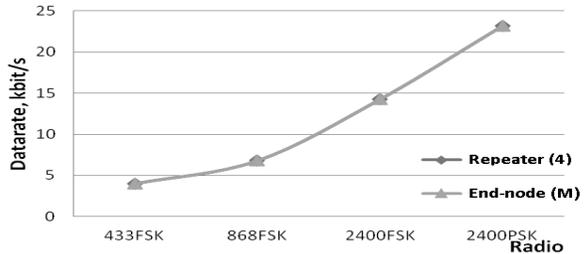
Figure 5. Maximum application data datarate for different radios over two hops in industrial environment (nodes C->4->M on Fig. 1)
