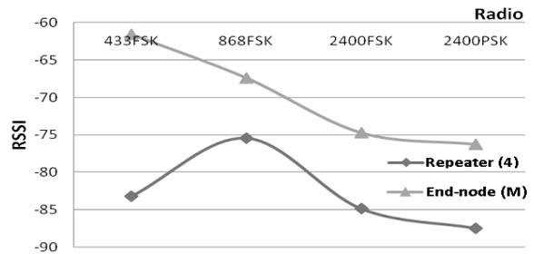
Figure 6. RSSI for different radios during two hop measurements in industrial environment (nodes C->4->M on Fig. 1)
