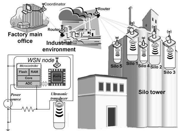
Figure 7. Structure of deployed IWSN for silos monitoring and structure of WSN node for silo level monitoring
