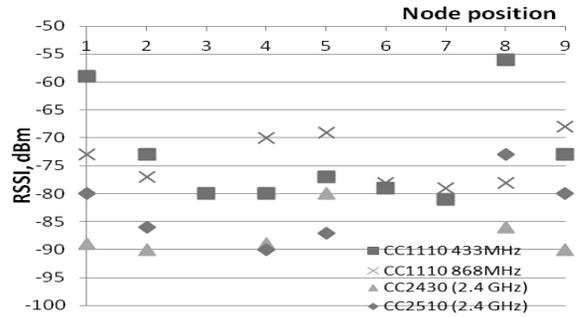
Figure 4. RSSI for signal from Coordinator(C) at different test points of industrial site (see Fig. 1 for test points location)
