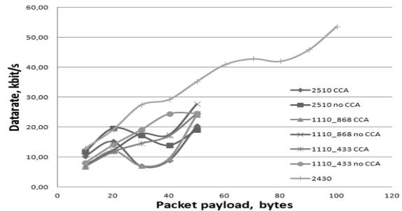
Figure 3. Maximum application data datarate for different radios over three hops in laboratory environment
