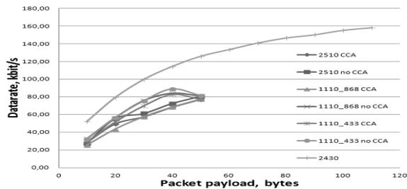
Figure 2. Maximum application data datarate for different radios over single hop in laboratory environment
