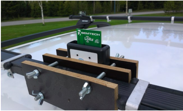
Fig. 1. The LoRa node mounted on the roof-rack of a car.
