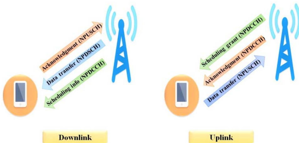
FIGURE 6-10 NB-IoT uplink/downlink transmission mode.
