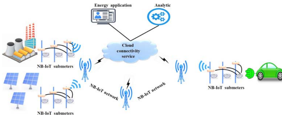
FIGURE 6–16 Smart vehicles charging-based NB-IoT infrastructure.
