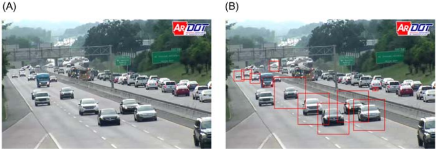
FIGURE 16-6 Traffic camera and cascade-based car detection algorithm. Figure (A) shows a snapshot of a traffic camera in Arkansas, United States, and figure (B) shows a traditional cascade-based detection algorithm only able to detect some of the cars. Data from https://www.kasu.org/post/arkansas-begin-streaming-nearly-100-traffic-cameras-online .
