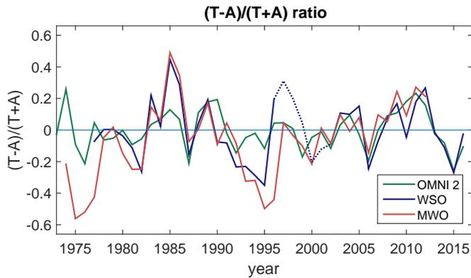
**Fig. 4.**  $(T - A)/(T + A)$  ratio measured with OMNI data (green) and predicted using WSO (blue) and MWO (orange) synoptic maps. The erroneous WSO times have been plotted with a dotted line.
