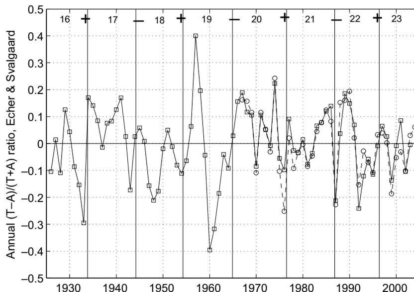
Fig. 2. Annual  $(T - A)/(T + A)$  ratios according to ES data (solid line with squares) and OMNI data (dashed line with circles). Plus and minus signs denote the solar polarity and numbers indicate the solar cycle number. Vertical lines denote the NGDC sunspot minima (Hiltula and Mursula, 2006).
