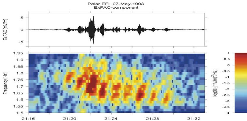
Fig. 7. Waveform and spectrogram of Polar electric field ( $x$  FAC-component) on May 7, 1998. The data are band-pass filtered over the wave frequency range at 1.5–2.0 Hz.
