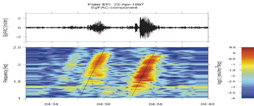
Fig. 8. Waveform and spectrogram of Polar electric field ( $x$  FAC-component) on April 23, 1997. The data are band-pass filtered over the wave frequency range at 1.0–2.5 Hz. The inclined lines are best fits to spectra in order to better depict the overall dispersion.
