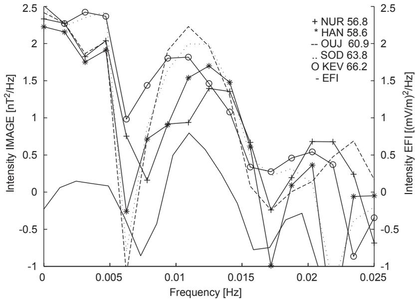
Fig. 4. Power spectra of Polar electric field (EFI) FAC  $x$ -component (solid line) and of the  $H$ -component of several Finnish IMAGE magnetometer stations in April 25, 1997, at about 0920 UT (Mursula et al., 2001). Dipole latitudes of each station are noted.
