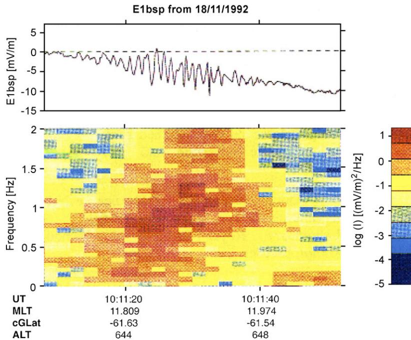
Fig. 2. Wave form and color coded spectral density of a dispersive Pc 1 pearl observed by the Freja electric field E1 component (magnetic field direction in spin plane) in November 18, 1992 (Mursula et al., 1994b).
