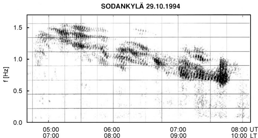
Fig. 1. Dynamic spectrum of a versatile Pc 1 pearl event observed at Sodankylä, Finland, in October, 29, 1994. Note the random, non-systematic variation of dispersion and the joining and separation of the different pearl bands.
