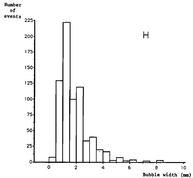
Fig. 2. The distribution of the width of the *H* component over the whole data period. The *x* axis gives the width in steps of 0.5 mm, and the *y* axis gives the corresponding number of *H* component chains with the largest bubble width in that interval. The average width is 1.7 mm.
