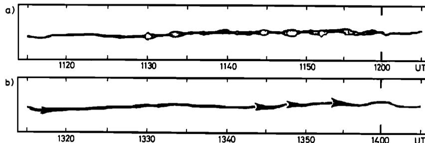
Fig. 1. (a) A typical example of a chain bubbles registered by the Sodankylä quick-run magnetometer system. (b) The nonmicropulsational background mainly consists of the clearly distinguishable arrow-head or wedge-shaped formed signals caused by thunder.
