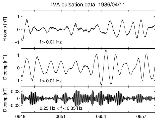
**Figure 2.** Search-coil magnetometer data from the IVA station during the Viking Pc 1 event. The two upper panels show the Pc 3 waves in the two components (DC trend has been removed); the bottom panel shows the the ground Pc 1 waves in the frequency range of the first Viking Pc 1 region.
