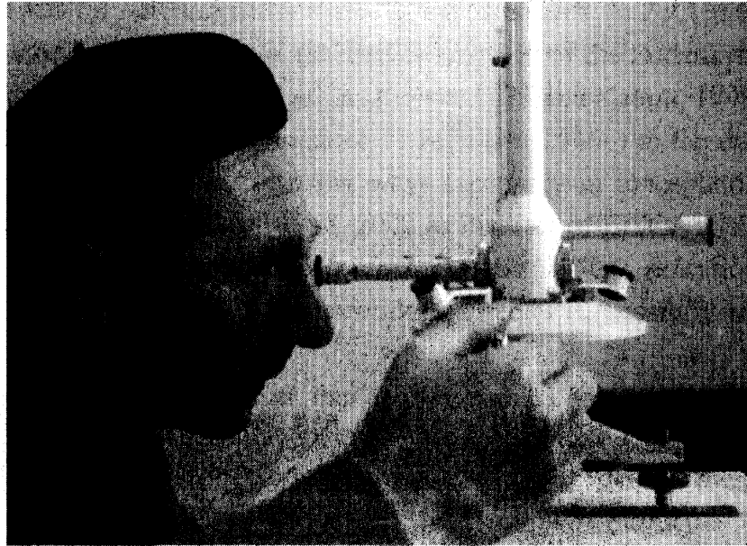
Fig. 3. Eyvind Sucksdorff (1899–1955), director of the Sodankylä Geophysical Observatory 1927–1944, here making absolute measurements with the Danish QHM-instrument. (Photo by C. Sucksdorff, FMI photoarchives.)
