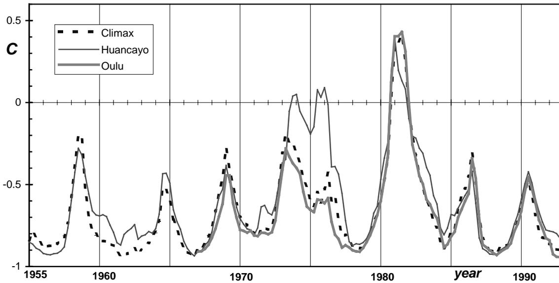
Figure 3. Coefficient of running-cross correlation between SA and CR for monitors with different geomagnetic cut-off rigidities: Huancayo (13 GV), Climax (3 GV), Oulu (<1 GV)
