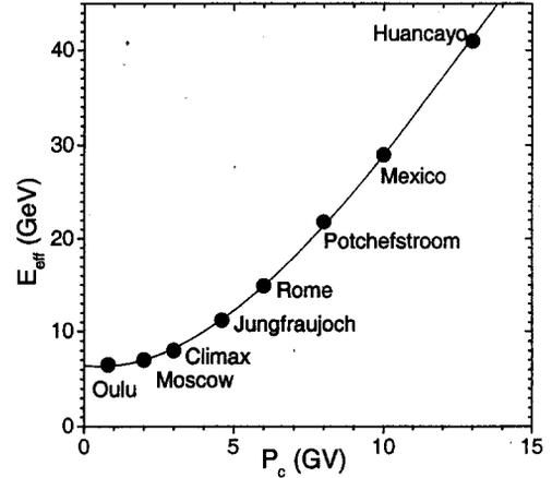
Fig. 4. The effective energy of a neutron monitor as a function of the geomagnetic rigidity cutoff. Dots correspond to some neutron monitors around the Globe (see Table 1).
