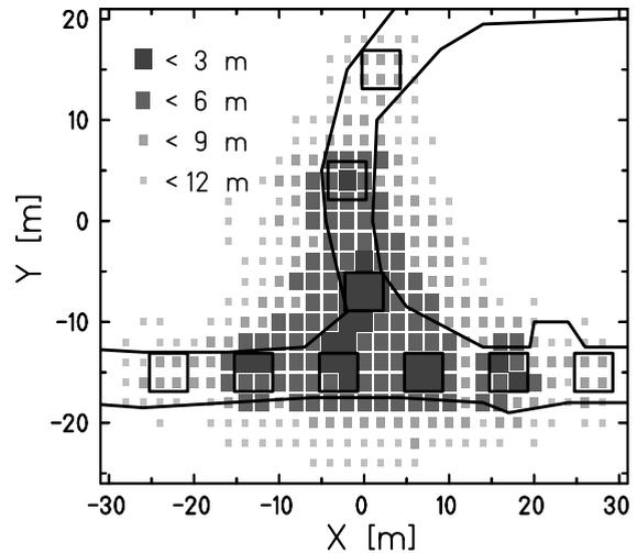
Figure 2. The accuracy of the reconstructed shower axis is shown as a cluster plot for a 4-PeV proton shower. The symbols represent the average shower axis uncertainty. The area where the shower axis can be determined with an average accuracy better than 6 metres is approximately  $300 \text{ m}^2$ . Each cluster contains 300 showers.
