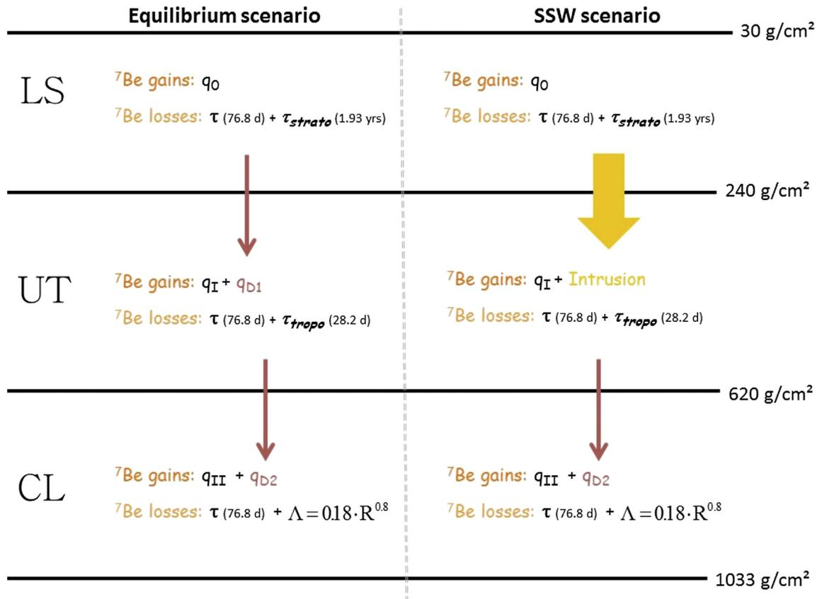
Fig. 3. Three-layer (LS – low stratosphere; UT – upper troposphere; CL – convective layer) numerical model for  $^7\text{Be}$  atmospheric deposition considering the normal equilibrium scenario (left) and the disturbed scenario for the SSW period (right).
