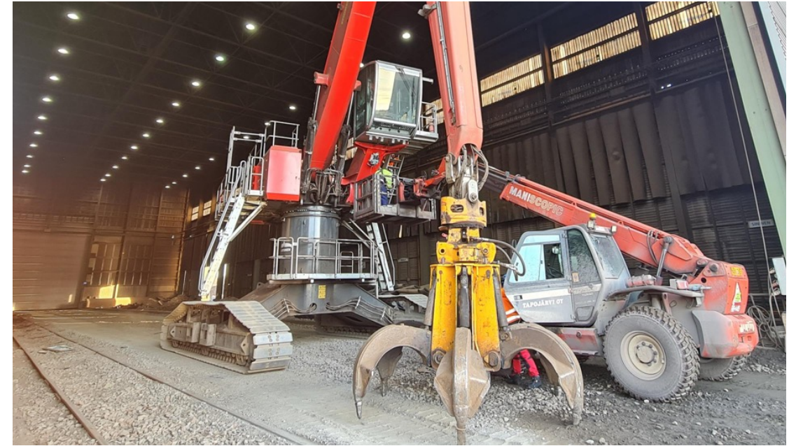
FIG 28 Mounting the portable sensor system on a Mantsinen 70R material handler.
