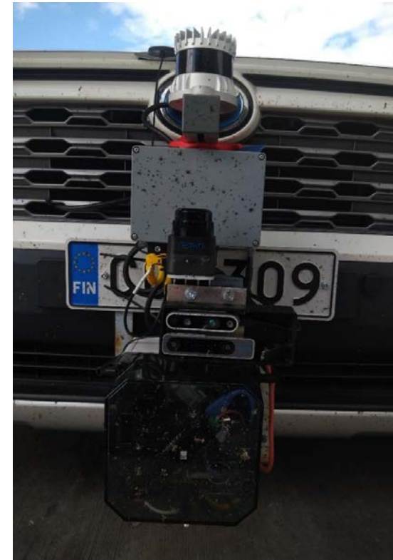
FIG 24 Portable sensor system mounted on the front of a car.
