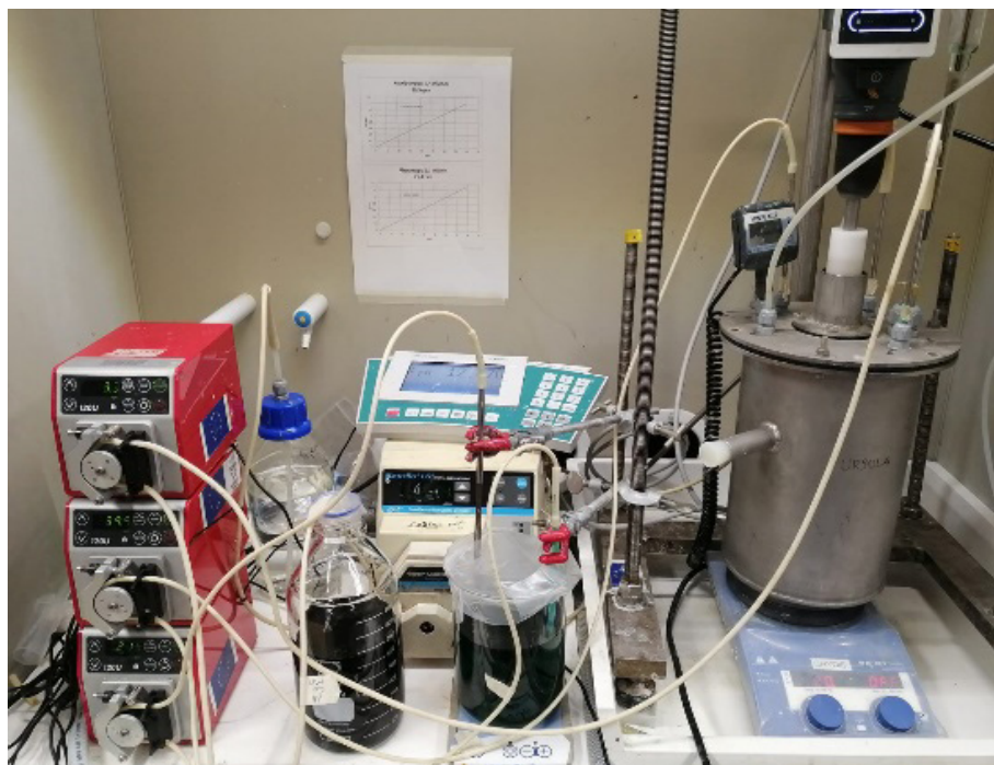
Figure 43. Precipitation reactor. Also autoclave precipitations were done.
