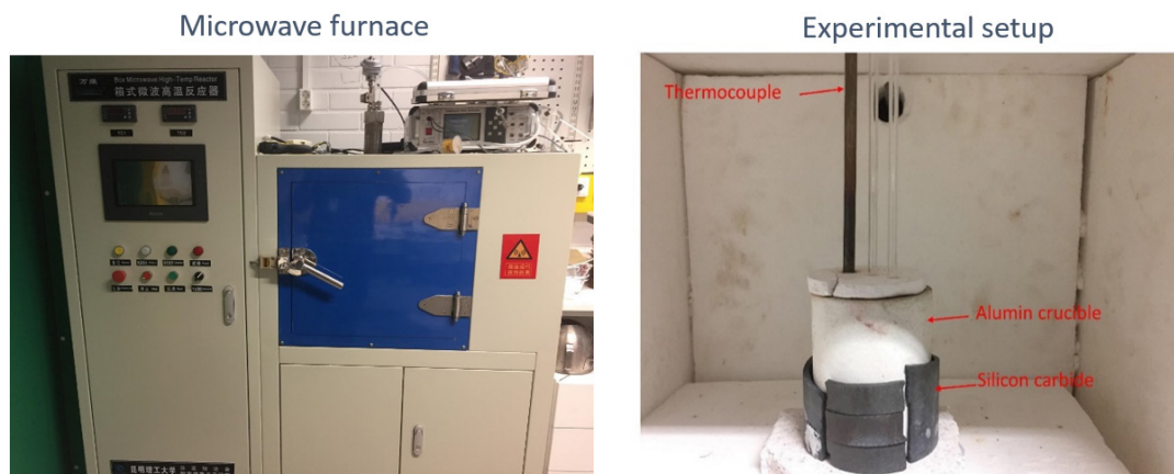
Figure 15. Experimental setup for microwave treatments.
