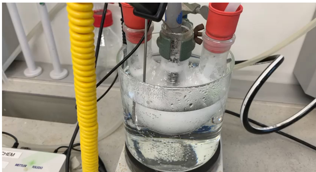
Figure 58. Reactor for CO 2 precipitation experiments.
