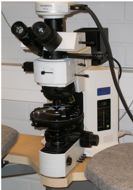
Figure 20. Olympus BX51 light optical microscope with camera was used in the study.
