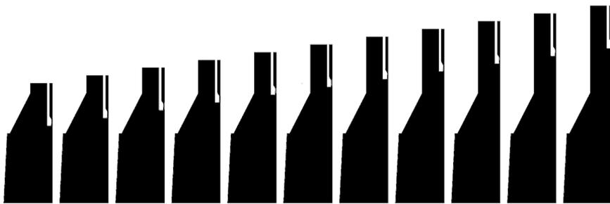
Fig. 11. All geometries for CFD modelling, with lance heights from 1 m to 2 m (modified from Paper III © 2015 Wiley-VCH).
