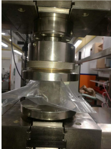
Fig. 6. Briquette placed between two parallel platens in 100 kN Zwick/Z100 machine used to perform compression strength tests for briquettes.
