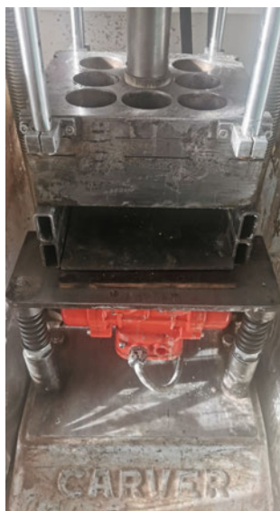
Fig. 5. A lab-press and die briquetting machine used to produce briquettes.
