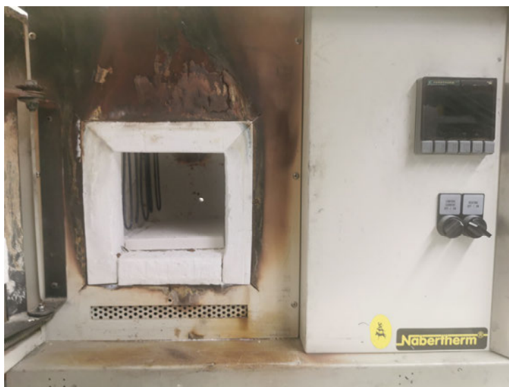
Fig. 9. Chamber furnace used to carry out melting trials for briquettes assessed for their suitability for EAF use.
