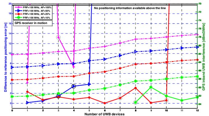
Figure 7. Difference to the reference positioning error, PRF = 100 MHz.
