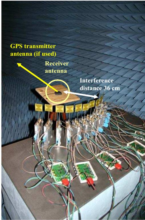
Figure 4. GPS measurement setup.
