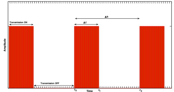
Figure 2. Burst like UWB transmission and parameters to calculate AF.
