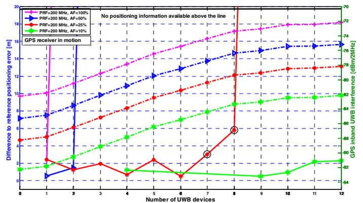
Figure 8. Difference to the reference positioning error, PRF = 200 MHz.
