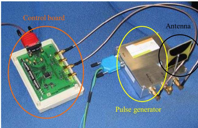
Figure 1. Prototype singleband UWB control board, pulse generator and antenna.
