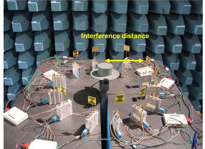
Figure 5. Aggregate noise measurement setup.
