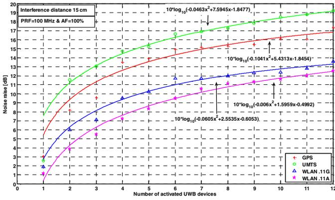
Figure 9. Aggregate noise raise as a function of the number of active UWB devices. PRF = 100 MHz and interference distance 15 cm.
