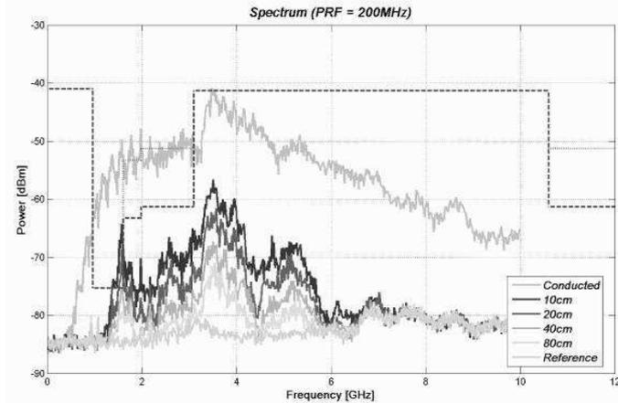
Figure 3. Spectra of the prototype UWB device.
