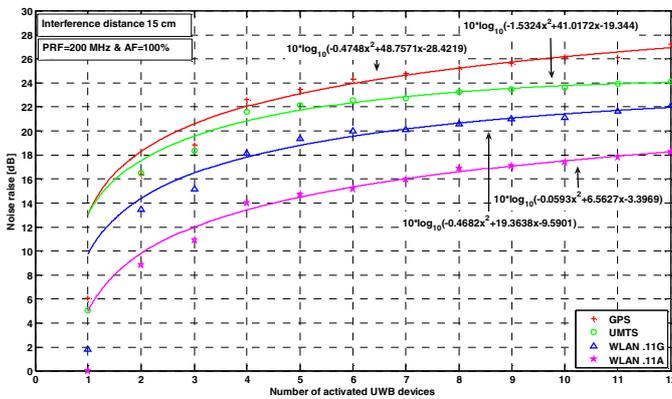
Figure 10. Aggregate noise raise as a function of the number of active UWB devices. PRF = 200 MHz and interference distance 15 cm.
