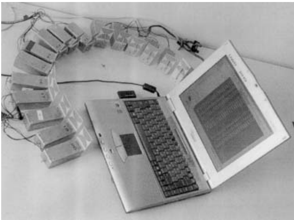
Fig. 3. UWB transmitters and WLAN receiver presented as used in a typical measurement setup.
