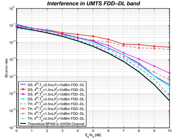
Fig. 5. BER for DS-UWB and TH-UWB systems utilizing the 4<sup>th</sup> derivative of the Gaussian pulse as a waveform with different pulse widths.
