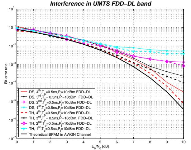
Fig. 4. UWB system performance degradation for different pulse waveforms when the jamming source is UMTS FDD-DL.
