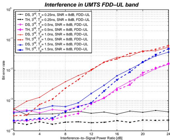
**Fig. 7a.** Bit error rate versus jamming-to-signal power ratio for different pulse widths. SNR = 8 dB and the jamming is in FDD-UL band. The UWB pulse waveform is the 3<sup>rd</sup> derivative of the Gaussian pulse.
