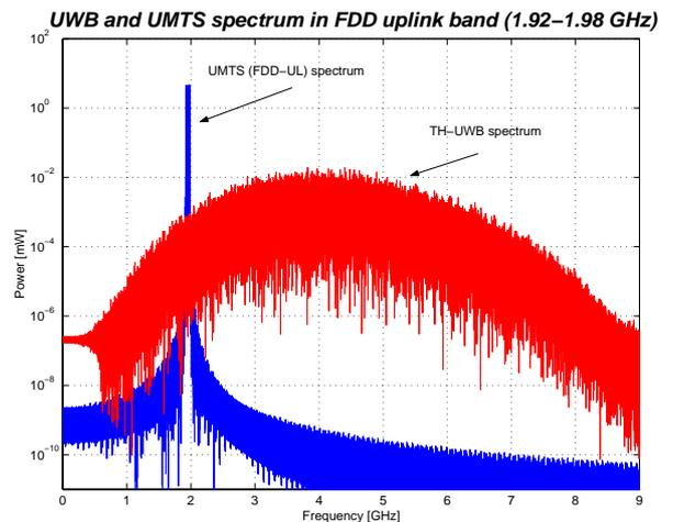
**Fig. 3.** Spectra of fully loaded UMTS FDD uplink band and UWB signal using the 3<sup>rd</sup> derivative of the Gaussian waveform.
