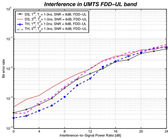
**Fig. 6a.** Bit error rate versus jamming-to-signal power ratio for the 1<sup>st</sup> and the 3<sup>rd</sup> pulses. SNR = 8 dB and the jamming is in FDD-UL band.
