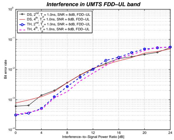
**Fig. 6b.** Bit error rate versus jamming-to-signal power ratio for the 2<sup>nd</sup> and the 4<sup>th</sup> pulses. SNR = 8 dB and the jamming is in FDD-UL band.
