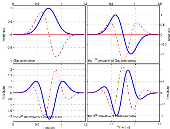
**Fig. 1.** The pulse waveforms used in the study. The solid lines represent the generated pulse waveforms and the dashed lines the radiated ones.
