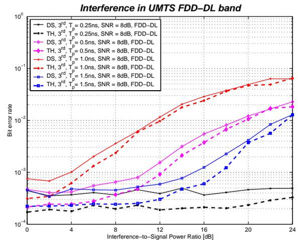
**Fig. 7b.** Bit error rate versus jamming-to-signal power ratio for different pulse widths. SNR = 8 dB and the jamming is in FDD-DL band. The UWB pulse waveform is the 3<sup>rd</sup> derivative of the Gaussian pulse.
