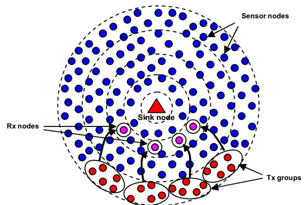
Fig. 1. UWB network divided into rings. The data flow from Tx groups towards the sink node.
