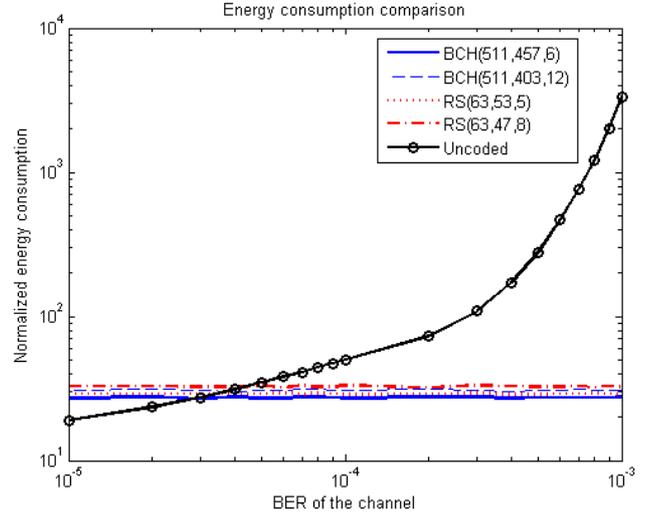
Fig. 4. Energy consumption; uncoded and coded cases.
