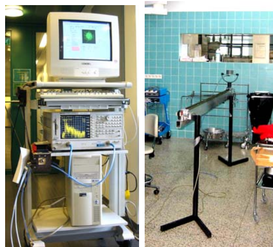
Figure 1. The measurement setup: a trolley and the antenna on the carriage.
