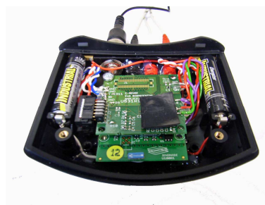
Figure 2: ExG amplifier board
