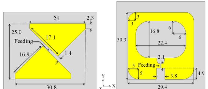
Figure 1. The CST simulation models of the planar UWB antennas (with TRF-43 antenna substrate) for the investigations: bow-tie dipole (left), and loop (right) antenna.
