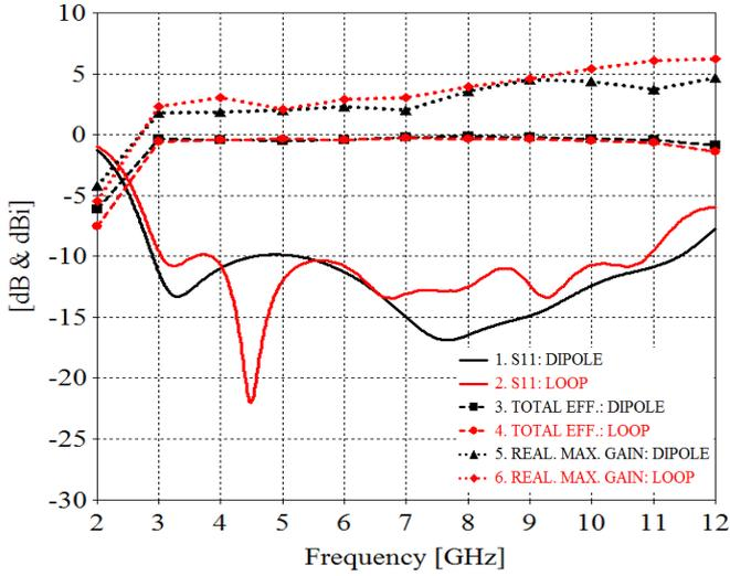
Figure 2. FS simulation results for investigated antennas: reflection coefficient  $S_{11}$  [dB], total antenna efficiency [dB], and realized maximum gain [dBi].
