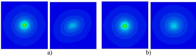
Figure 3. Temperature distribution in  $xy$ -plane for a) dipole and b) loop antenna with different tissue models, when *PIP* of 50 mW is fed to the antenna: M1 (left), and M2 (right). Temperatures are scaled such that 36.0 °C corresponds to blue, while red for 37.0 °C. In each plot, cutting plane is aligned immediately below the antenna, at the top of tissue model.
