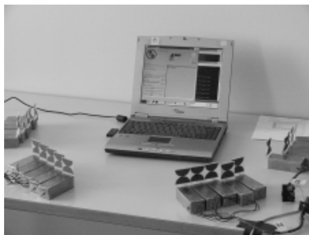
Figure 1. UWB transmitters and the example of the measurement setup.
