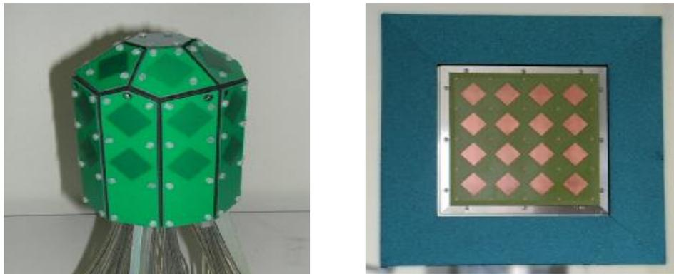
**Figure 2.** Dual-polarised antenna arrays for 5.25 GHz channel probing. The 3D antenna array on the left was applied as a transmit antenna and the 4x4 array on the right was used at the receiver.
