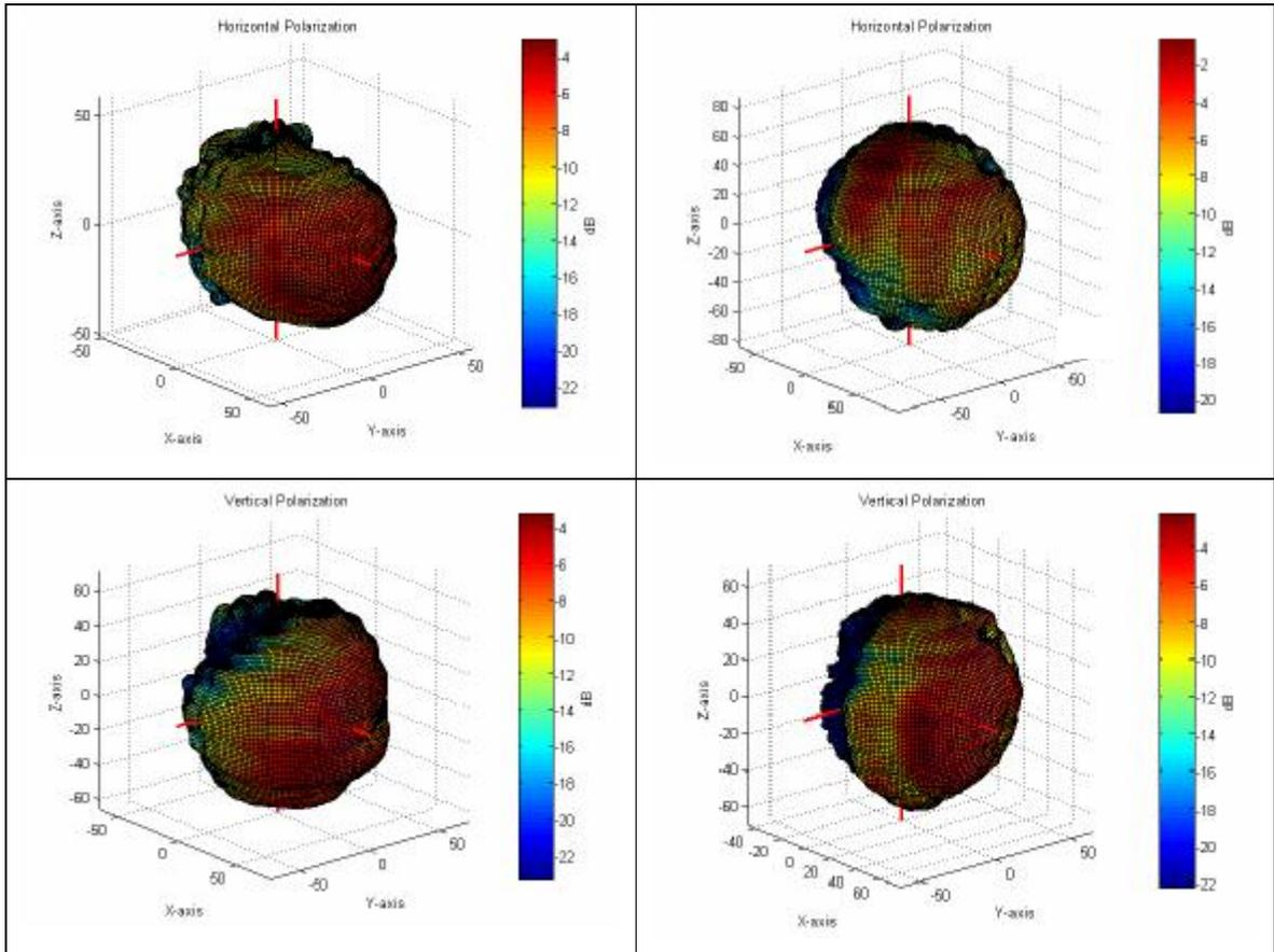
**Figure 3.** Normalized power patterns for the dual-polarised antenna arrays for 5.25 GHz channel probing (left column: TX antenna element, right column: RX-antenna element). Horizontal polarization is depicted on top row and vertical polarization on bottom row.
