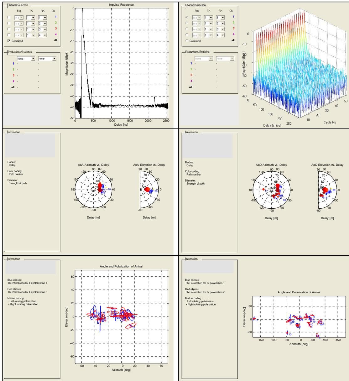
**Figure 5.** Impulse response measured in position 1 (LOS case, top left), waterfall representation of it (top right), angles of arrival in polar display (middle left), angle of departure (middle right), polarization (and angle) of arrival (bottom left), and polarization (and angle) of departure (bottom right).
