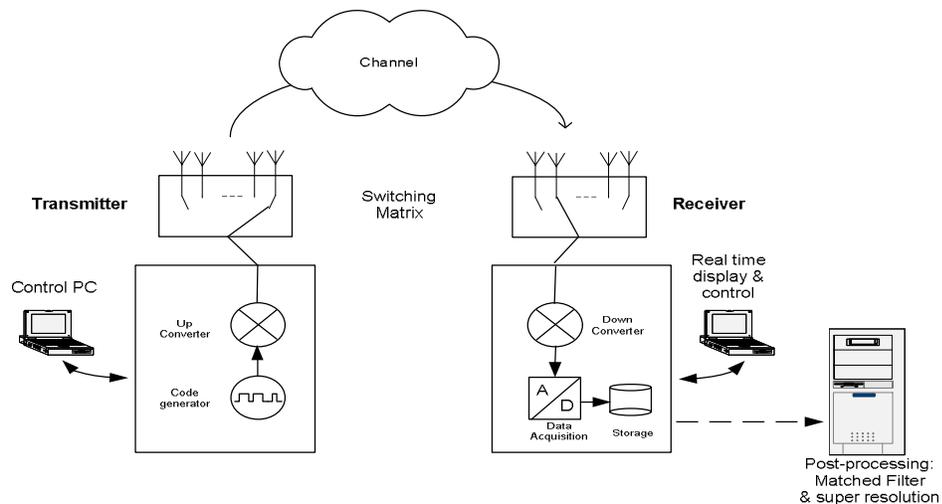
**Figure 1.** Block diagram of the multi-dimensional radio channel sounding system.
