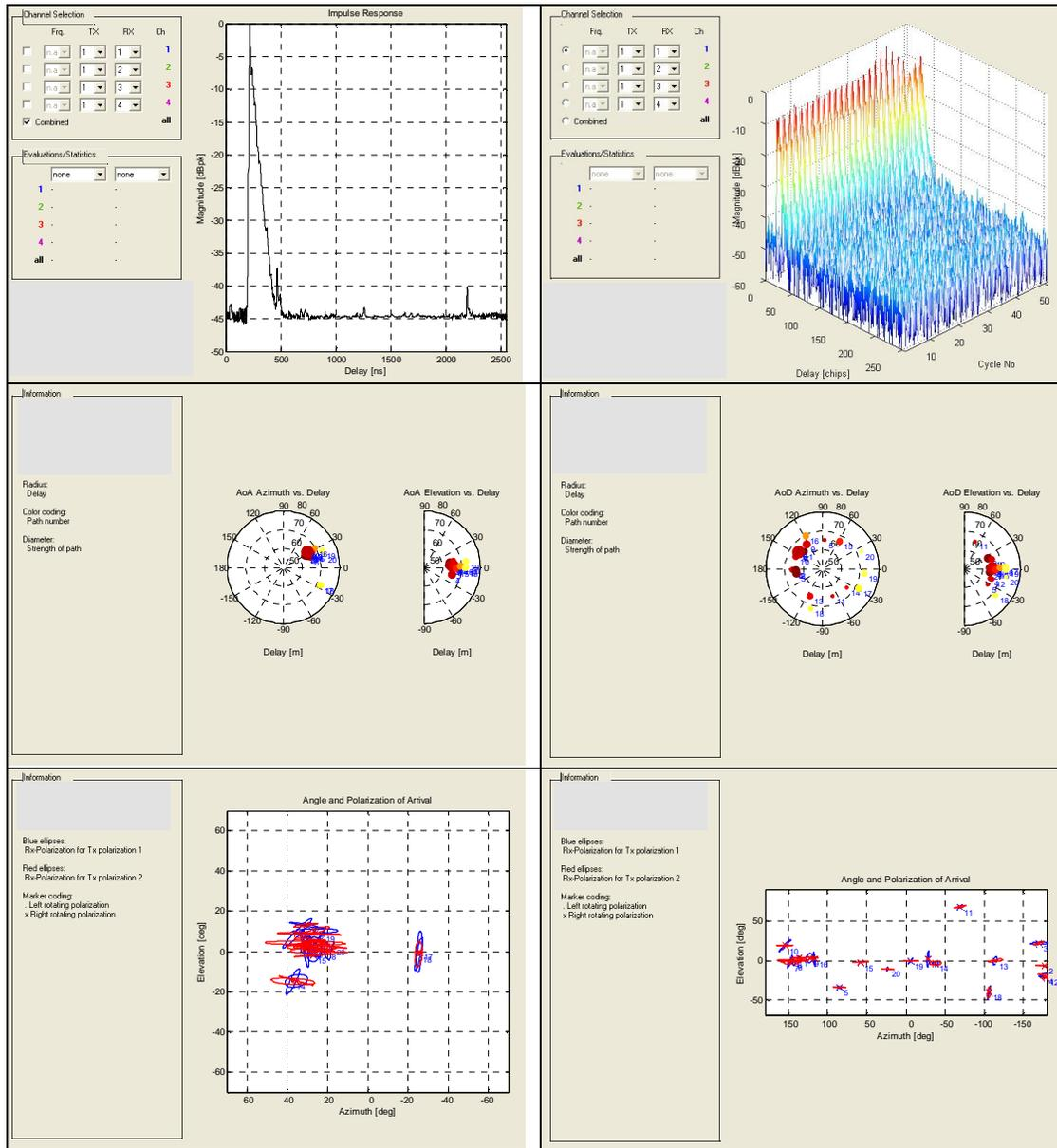
Figure 6. Impulse response measured in position 2 (NLOS case, top left), waterfall representation of it (top right), angles of arrival in polar display (middle left), angle of departure (middle right), polarization (and angle) of arrival (bottom left), and polarization (and angle) of departure (bottom right).
