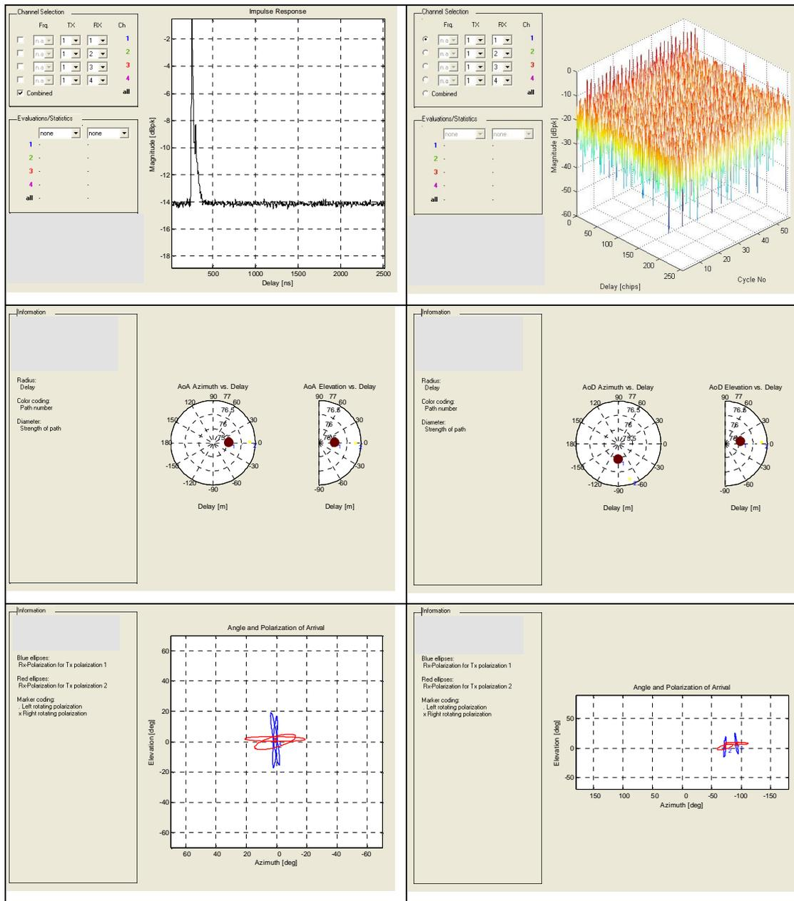
**Figure 7.** Impulse response measured in position 3 (NLOS case, top left), waterfall representation of it (top right), angles of arrival in polar display (middle left), angle of departure (middle right), polarization (and angle) of arrival (bottom left), and polarization (and angle) of departure (bottom right).
