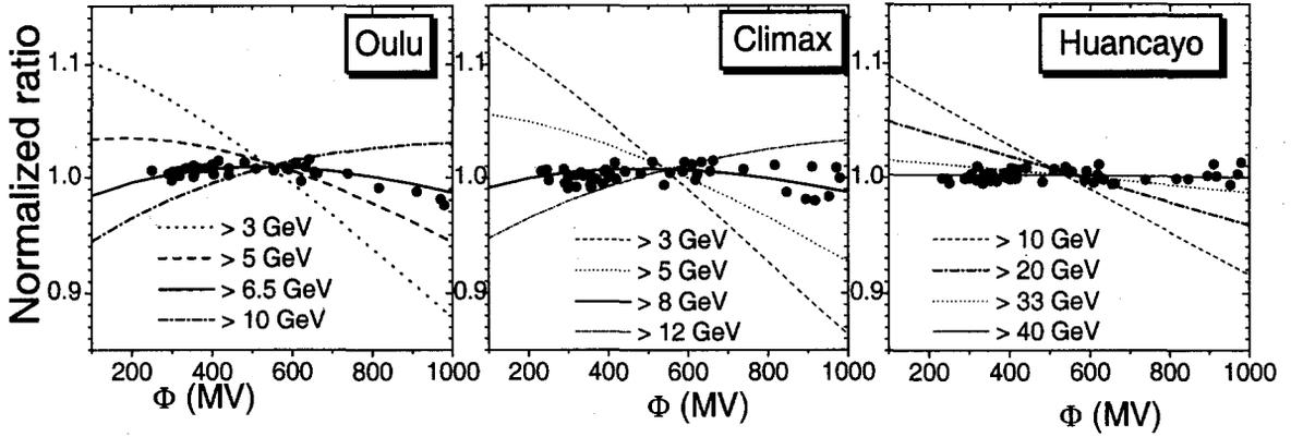
Fig. 2. Normalized ratios of the model calculated flux of GCR with energy above  $E_{eff}$  (as denoted in the legend) to the response of a neutron monitor, as a function of the modulation strength  $\Phi$ . Lines correspond to model calculations of the NM response, and dots correspond to the actual NM annual count rates. The neutron monitors are: Oulu (sea-level NM64,  $P_c = 0.8$  GV), Climax (mountain IGY,  $P_c \approx 3$  GV) and Huancayo (mountain IGY,  $P_c \approx 13$  GV).
