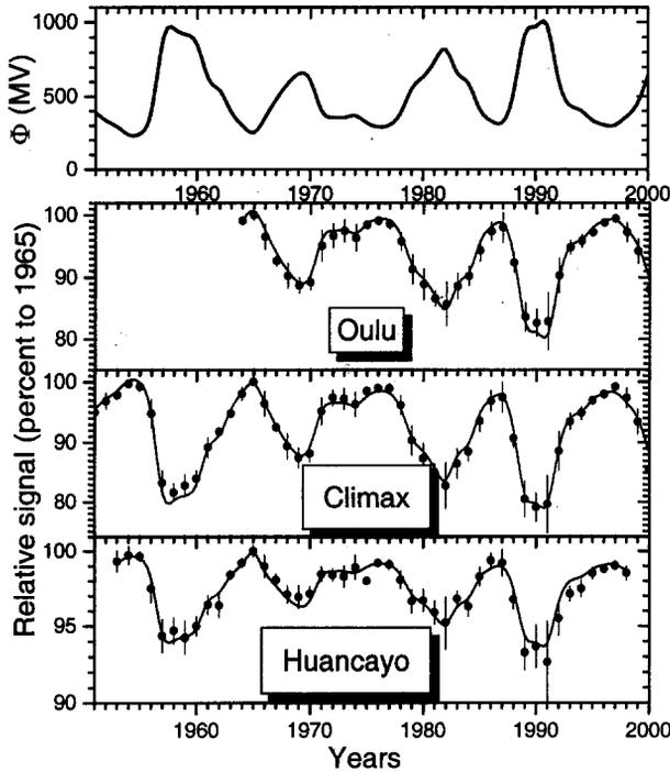
Fig. 3. Top panel: Annual modulations strength  $\Phi$ . Lower panels: Actual annual count rates of Oulu, Climax and Huancayo NMs (dots) and the calculated GCR flux with energy above 6.5 GeV, 8 GeV and 40 GeV, respectively, at the Earth's orbit (curve), in percent to the values in 1965. Error bars represent fluctuations of monthly values around the annual mean.
